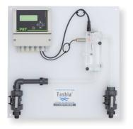
Pre-assembled system with PRT controller and pH electrode, with a long-term stable reference system with gel electrolyte and additional salt deposit to extend useful life.
