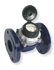
Turbine meters with hydrodynamically balanced rotor and symmetrical calibration adjustment. They have a broad measurement range with good resolution throughout the working range. Possibility to easily insert a pulse emitter.
