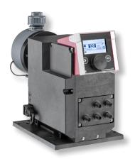
Digital membrane dosing pump, with a stepper motor and electronic stroke control and adjustment system with high turn-down ratio (1:800). Easy-to-use interface with pump performance displayed in I/h with perfect calibration, for improved use and unrivaled precision. Includes smart Auto-FlowAdapt feature with real-time pressure and flow rate control.
