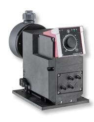
Constant/proportional membrane dosing pump, with a stepper motor and electronic stroke frequency system with a high turn-down ratio (1:800).
