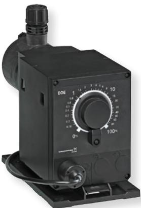
Constant/proportional membrane dosing pump, with a stepper motor and electronic stroke frequency system with a high turn-down ratio (1:1000).
