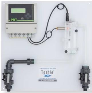
Pre-assembled system with PRT controller and pH electrode, with a long-term stable reference system with gel electrolyte and additional salt deposit to extend useful life.
