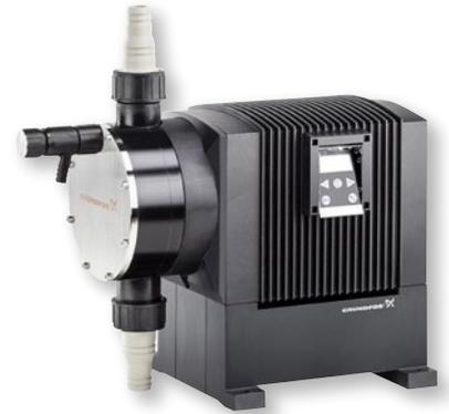
Constant dosing pump with manual adjustment from 10 to 100% of the nominal flow rate. Dosing ratio of 1:10.
