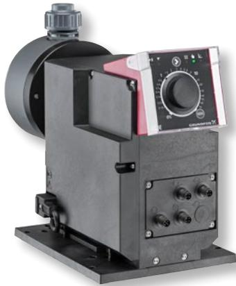
Constant membrane dosing pump, with a stepper motor and electronic stroke frequency system with a high turn-down ratio (1:800).
