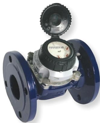
Turbine meters with hydrodynamically balanced rotor and symmetrical calibration adjustment. They have a broad measurement range with good resolution throughout the working range. Possibility to easily insert a pulse emitter.
