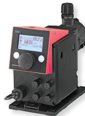
Digital membrane dosing pump, with stepper motor and electronic stroke control and adjustment system with a high turn-down ratio (1:1000). Easy-to-use interface with pump performance displayed in l/h with perfect calibration, for improved use and unrivaled precision.
