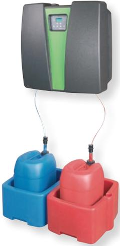
Automatic batch systems for the generation and application of chlorine dioxide in water, through the combination of chlorite and acid with proper dosing and mixing.
